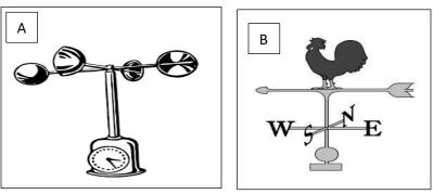
[Hint-A-anemometer -to measure wind speed; B- Wind vane -to find direction]
